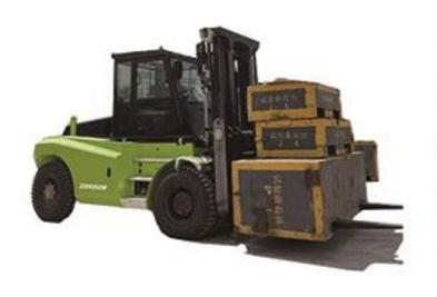
©USING SPEED LIMIT VALVE AND PRESSURE SELECTOR VALVE, REDUCE THE HYDRAULIC SYSTEM IMPACT, CAN LOWER THE MAST TO THE GROUND WHEN ENGINE FLAME OUT
